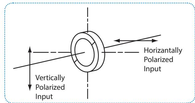
The change in phase due to the birefringence will be dependent on the plate thickness ( $d$ ) of the material, as well as, the wavelength ( $\lambda$ ) of the beam of incident light and the birefringence value. The resultant phase difference can easily be shown to be:
