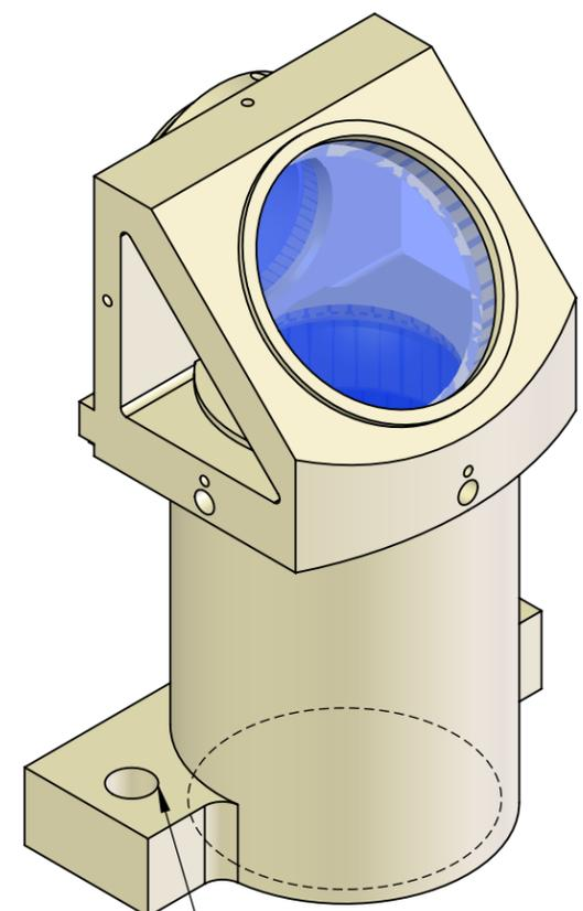
D CLEARANCE HOLES FOR 1/4-20 SCREWS
